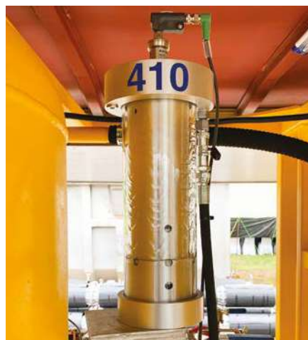
VZ212A applied on a VOP plant to measure water and total gas content
