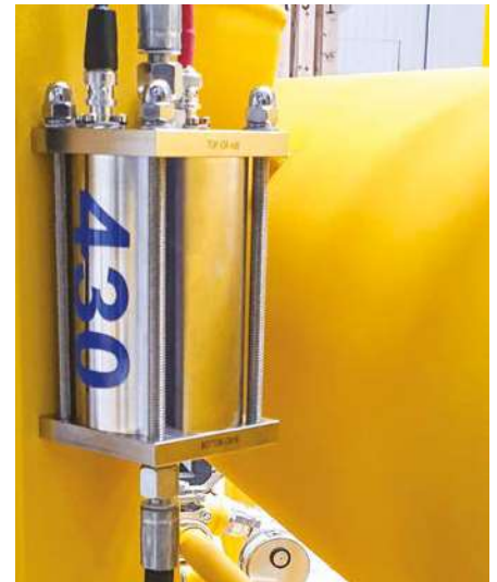
VZ220A applied on a VOP plant to measure Tan Delta
