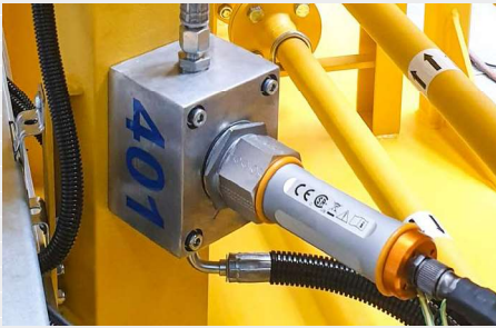
MicaSonic™ applied on a VOP plant to measure - Breakdown voltage [kV] - Moisture content [ppm] (@ 20°C and actual temperature as per IEC)
