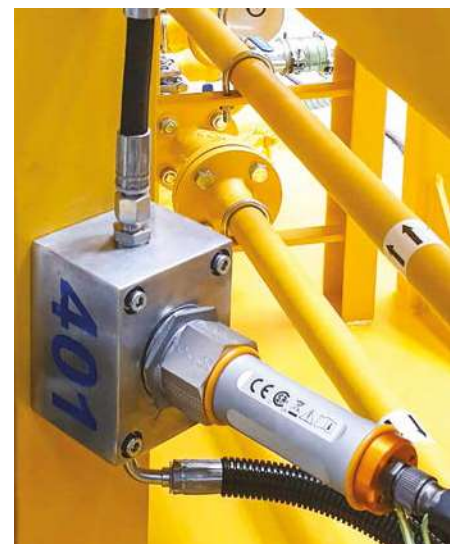
MicaSonic™ applied on a VOP plant to measure: - Breakdown voltage [kV] - Moisture content [ppm] (at 20 \text{ }^\circ\text{C} and actual temp. as per IEC)
